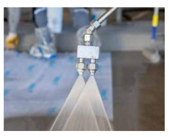
The double and a single nozzles are easy to interchange, and spare nozzles plus a nozzle extension are provided in addition. To prevent the nozzles from clogging with cured material after using Triflex SAM, they are placed in a container with Triflex cleaner, which is also supplied.
